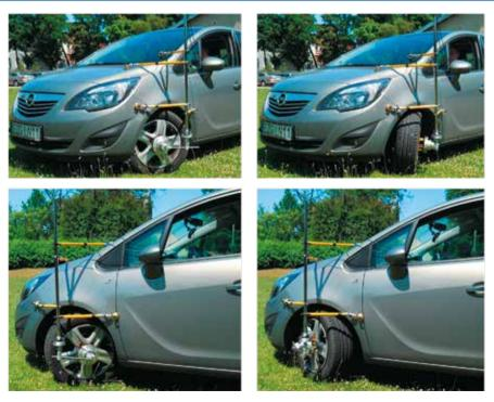
Fig. 7. View of the device mounted on a real car
